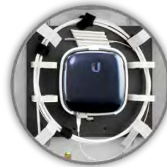
Slack storage for coiling up to 50 feet of fiber
